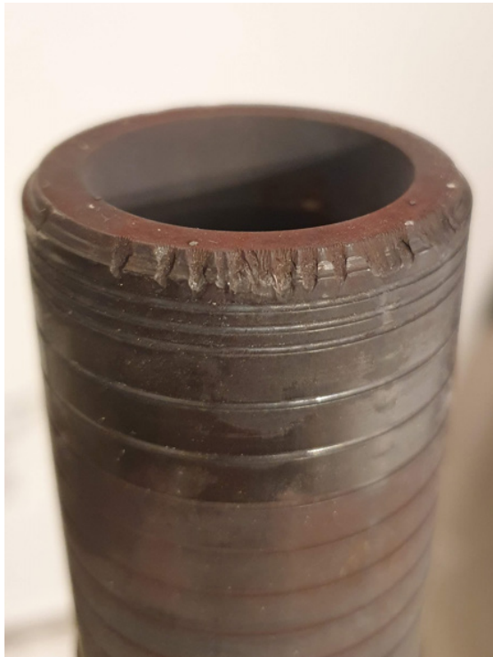
Figure 5 Cavitation damage on internal parts
