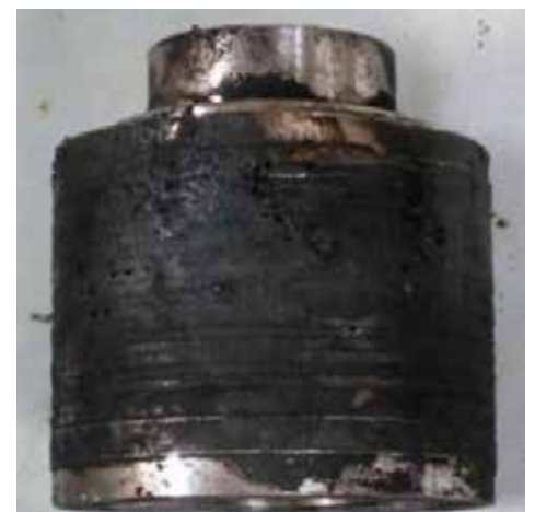
The original multistage valve trim clogged by sand and sticky fluid.
