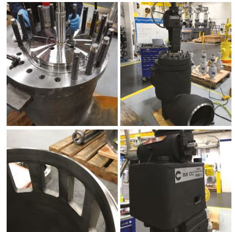
Clockwise (top left): Assembly showing piston rings on plug. Assembled valve. Gear locking mechanism. Cage valve trim.
