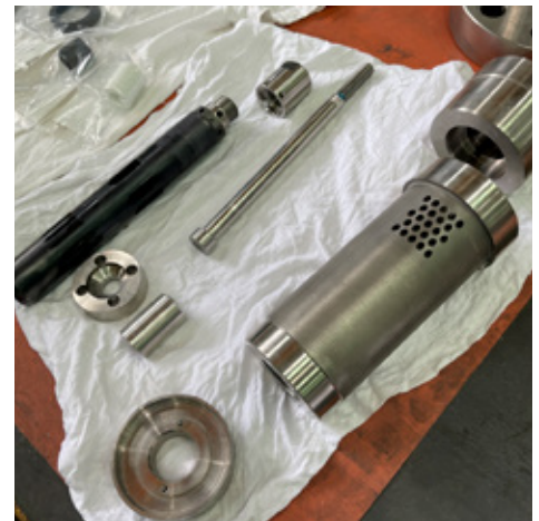
Figure 3: EroSolve MMT parts inspected after 3 months of service
