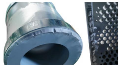
Erosion was present in the plug and cage.
