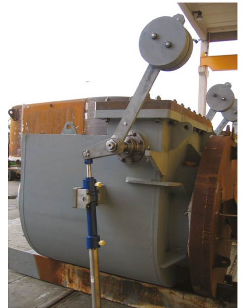
Check valve during a hot stroking test
